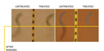
Anti-stain testing carried out on Vicenza Stone and terracotta. The untreated section absorbed the cement deep down, which made washing after laying difficult.
